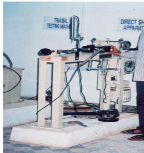
Fig.2 Direct Shear Test Apparatus
