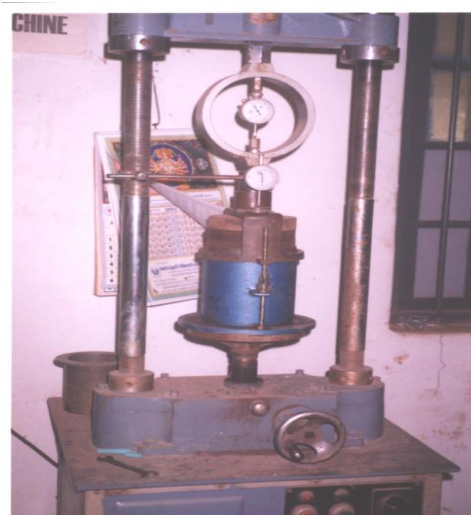
Fig.3 California Bearing Ratio Test Apparatus
