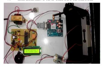
Weight of the chamber is estimated by utilizing load cell it is coordinated with arduinouno ESP8266 12E is IOT module to control the gadgets all segments are associated with arduniouno. Gas level is shown in LCD and we can ready to see it in android application. On the off chance that any release happens, at that point gas sensor detects spill and send an alarm message to the LPG gas client at that point fumes fan will be turned on promptly to keep away from significant mishaps.
