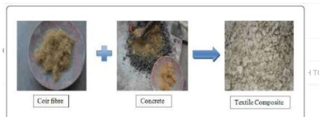
Fig: Coir fibre mixed with concrete as reinforcement
