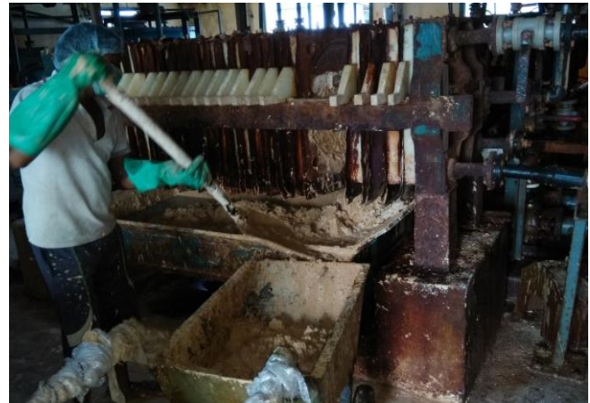
Fig(2). Filter tray, removing sulfur
