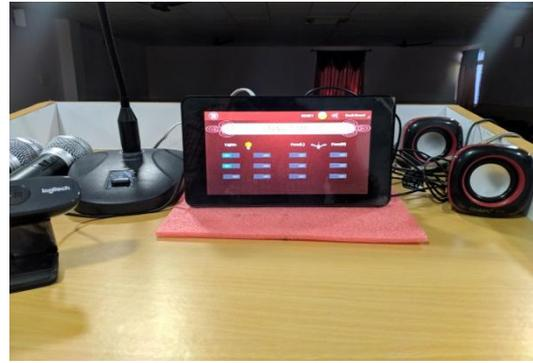
**Fig. 10 LCD touch screen and main control unit placed on the podium front view**
