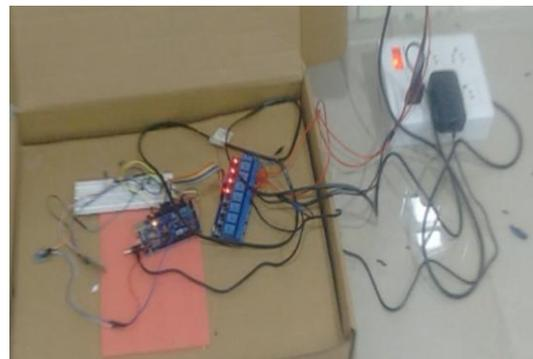
**Fig. 12 relay controlling unit having Arduino mega, Bluetooth module and relay module.**
