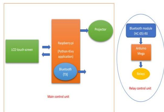
Fig. 1. Block diagram of conference halls automation scheme
