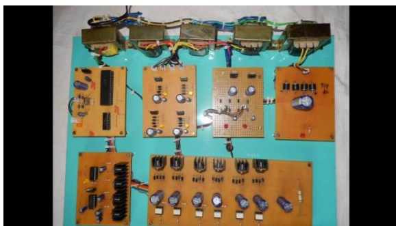
Fig 7. Experimental Setup Of 15- Level Inverter
