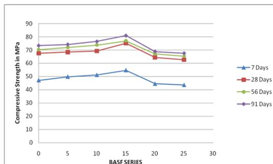
**Fig 1 Compressive Strength of TBASF Ternary Concrete**
