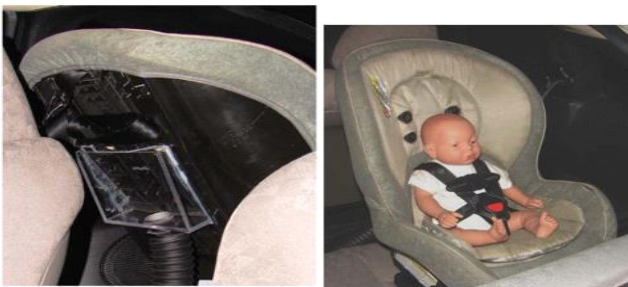
Fig. 4. Smart child safety seat with mannequin featuring an integrated cooling system for emergency elevated temperature scenarios.
