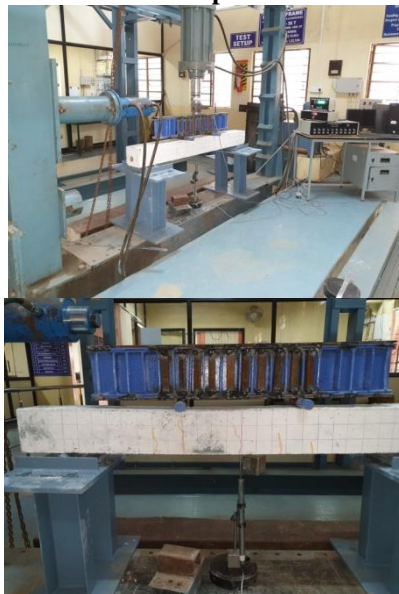
Figure 3 Failure form of composite beam and load setup
