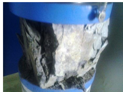
Fig.2 Test Specimen at Collapse
