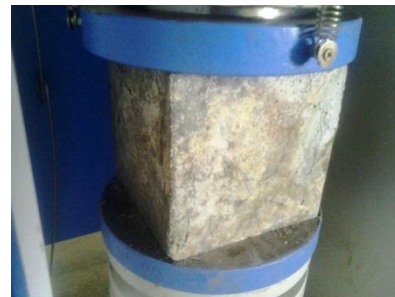
Fig.1 Test Specimen at Cracking
