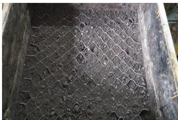
Fig.6. Filling GSB materials in rubber cell
