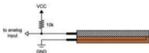
Fig 5. Voltage Driver (Flex sensor connection)
