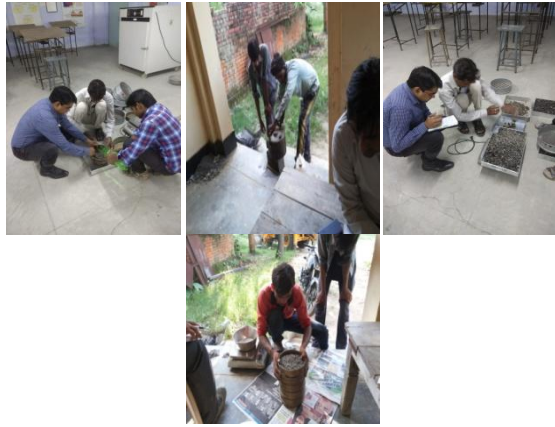
Fig 2: Washing, Extracting and Gradation Experiment of RAP
