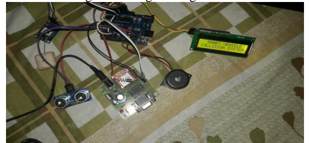
Fig.7. Hardware overview of smart vehicle accident collision detection system
