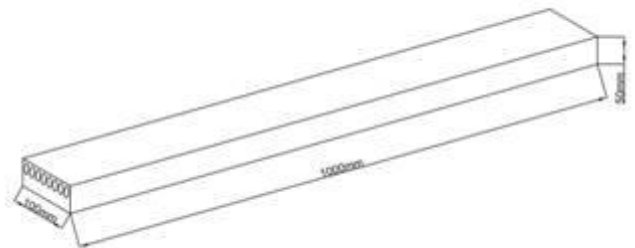
Fig.2. Beam With SMA
