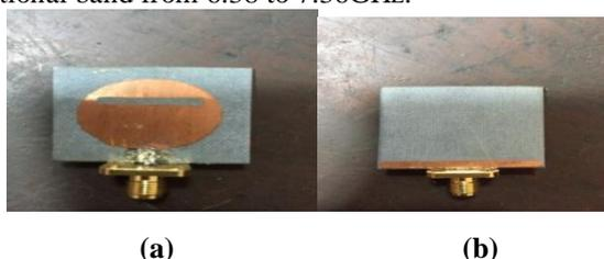
**Fig.7.** Fabricated antenna prototype (a) Front view (b) Rear view
