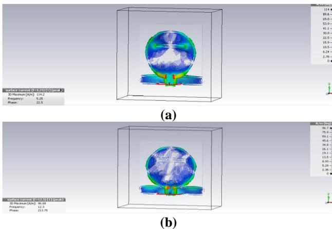
**Fig.3.** Surface Current distribution results for the suggested antenna
