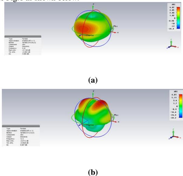
**Fig.6.** Directivity plot at (a) 5.25 GHz and (b) 12.3GHz.
