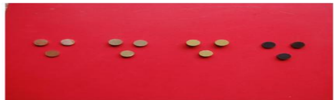
Fig: 8: heat treated sintered pellets at 550°C exposed in hydrogen atmosphere for 30 min minutes
