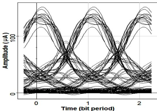
Fig.3 Eye-diagram with LiNbO<sub>3</sub> scheme at 110 km
