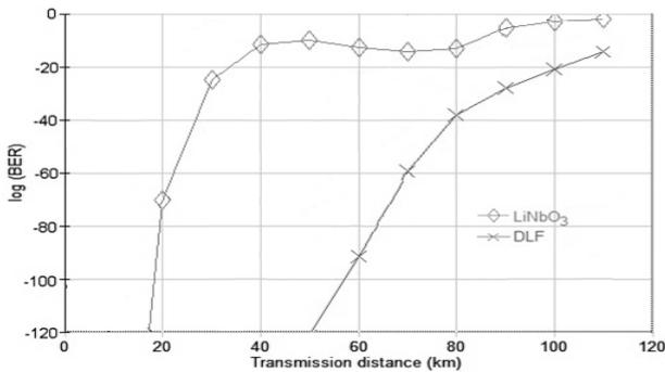
Fig.2 BER performance versus transmission distance
