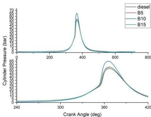
Graph 5 cylinder pressure Vs. crank angle.
