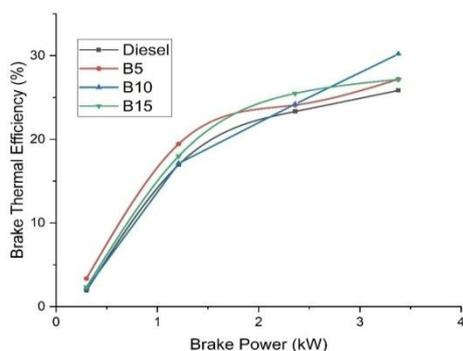
Graph 1 Brake power Vs. Brake thermal efficiency
