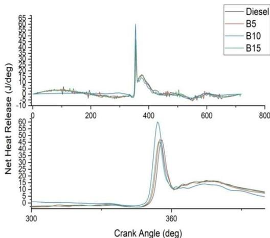
Graph 6 Net heat release Vs. Crank angle
