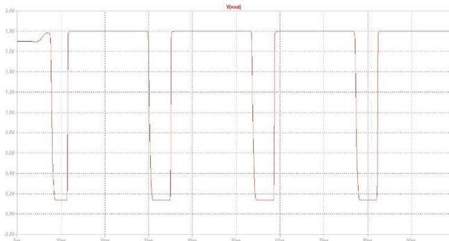
Fig (e)-5 stage VCO output with conventional BGR
