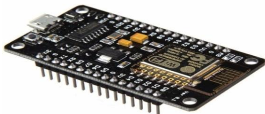
Figure: 2 Structure of NodeMCU
