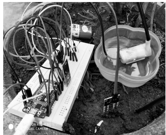
Fig.13 Soil Moisture Monitoring System set-up
