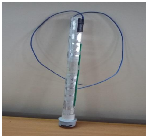
Figure 4: Experimental setup with capacitive sensor arrangement
