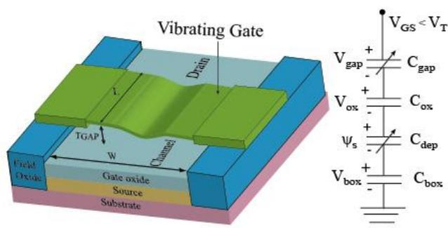
Fig: 2 3D Design for single gate(SG-FET) MEMS microphone
