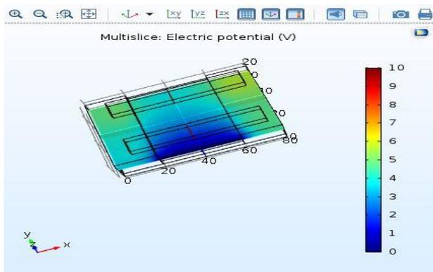
Fig: 7 DG –MOSFET at 10V
