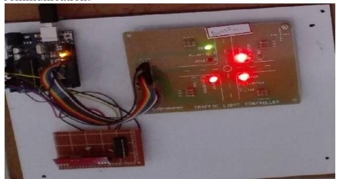
Fig 6: traffic signal changed based on the input from ambulance transmitter
