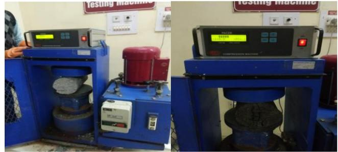
Fig. shows the split tensile testing on cylinders.
