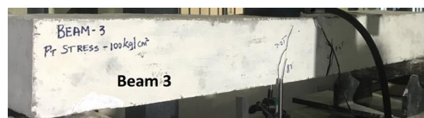
Fig.4d Crack patterns in specimen 3
