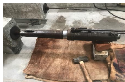
Fig.2 Application of prestressing force to beams
