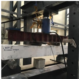
Fig.3a Test setup of beam for two point loading
