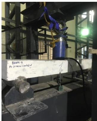
Fig.3b Test setup of beam for single point loading
