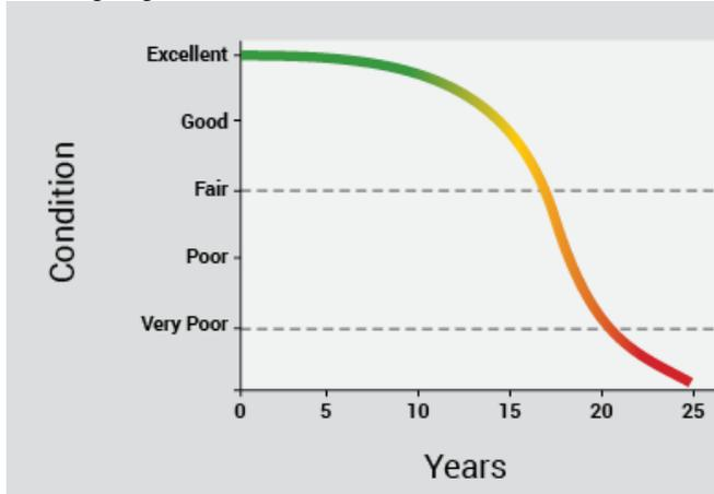
**Fig. 1 The building condition level over the life cycle**
