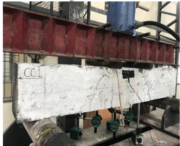
Fig 5 RCC Flexural Beam Testing Arrangements
