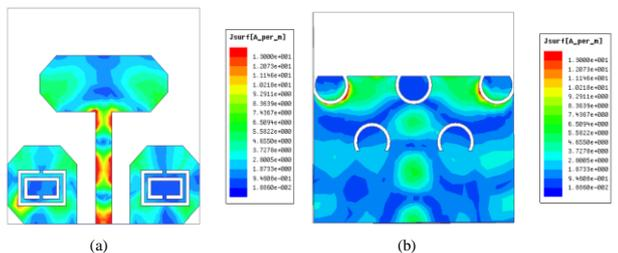
**Fig.5** Current distribution at 37 GHz
