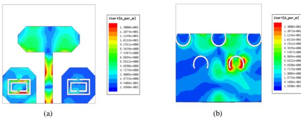
**Fig.4** Current distribution at 28 GHz
