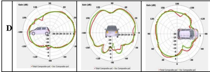
Table 2. represents the antenna placed on the different position of the car at the 5G communication band i.e., at 28GHz. The observation of the radiation in the vehicular region mainly depends on the placement of the antenna in vehicular area. The radiation stableness in the car is almost same with variance of the position.
