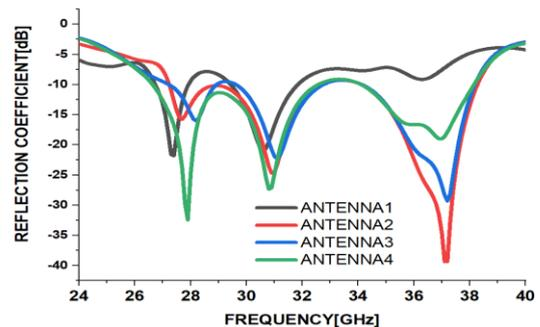
**Fig.2** Reflection coefficient of all the iterations.
