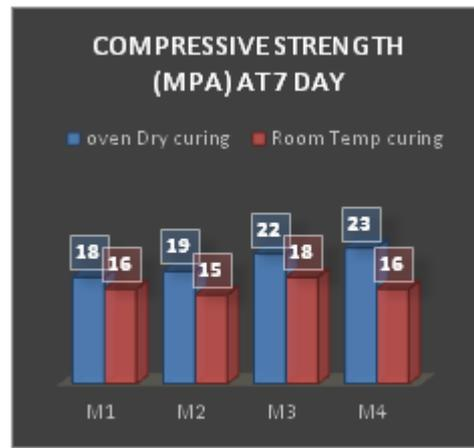
Figure 2. Compressive Strength (Mpa) at 7 Days
