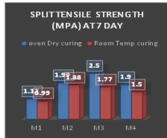
Figure 6. Split Tensile Strength (Mpa) at 7 Days.
