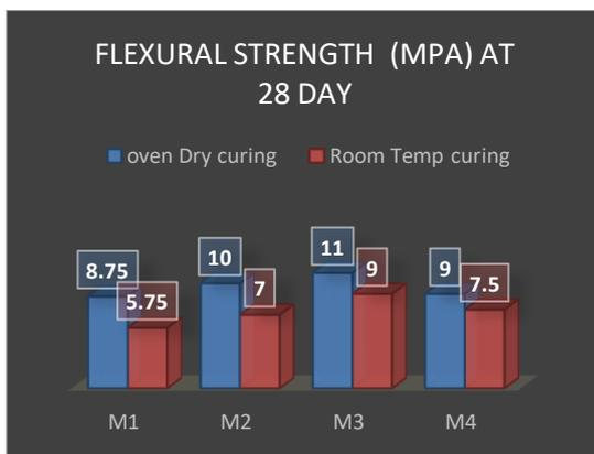
Figure 5. Flexural Strength (Mpa) at 28 Days.
