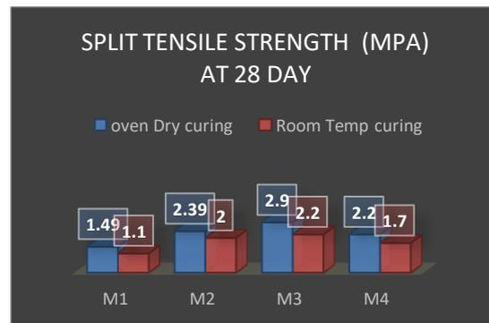
Figure 7. Split Tensile Strength (Mpa) at 28 Days.
