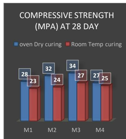
Figure 3. CompressiveStrength (Mpa) at 28 Days.
