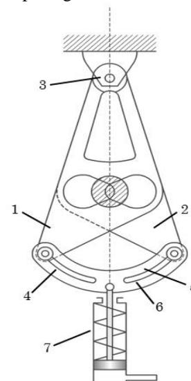
Fig. 1. Schematic view of the control valve: 1, 2 – plates, 3 – axle, 4, 5 – guides, 6 – cam, 7 – linear drive.
