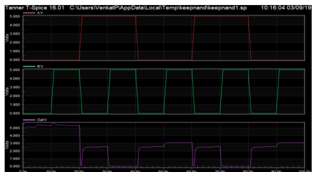
Fig8: The above figure is about sleepy keeper method with nand gate output graph.
