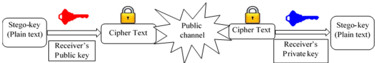
Fig. 5: Stego-key encryption, transmission, and decryption using public key cryptography
