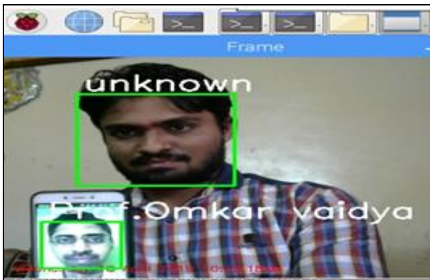
Fig. 8 Face Recognition for tagged face in dataset and another unknown face using LBPH Algorithm
