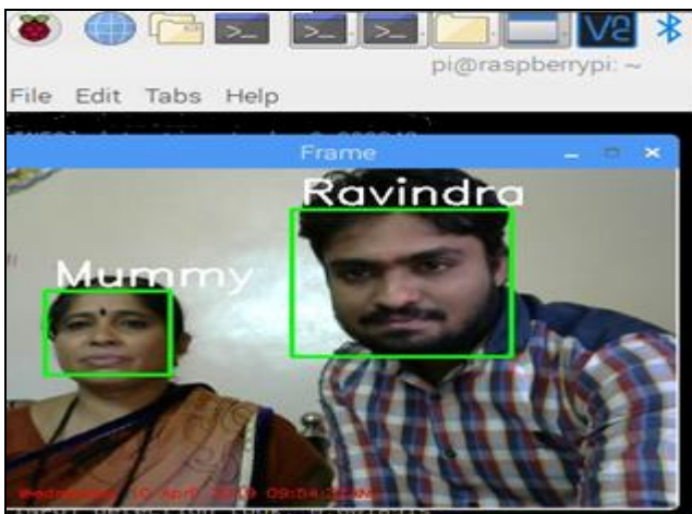
Fig. 9 Face Recognition for both tagged faces in dataset using LBPH Algorithm
