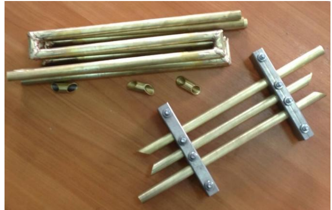
Fig. 2. Samples of condenser piping prepared for soldering (a) and already soldered (b).
