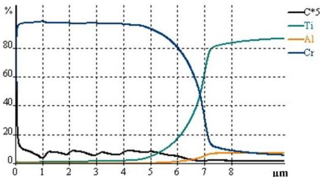
Fig. 10. Changes in the elemental composition over the depth of the surface layer of the Ti6Al4V titanium alloy with Cr-CrC coating
