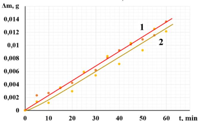
Fig. 13. Results of solid particle erosion tests of compressor blades without the coating (1) and with the coating (2) (the tests on the convex side)
