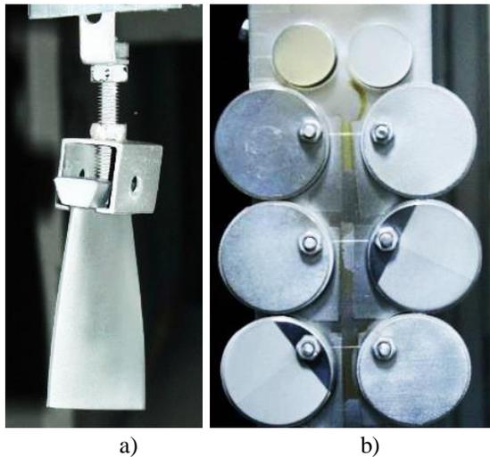
Fig. 4. Part of the compressor blade (a) and the experimental samples (b), mounted on the technological equipment of the vacuum chamber of the "Gefest+" installation
