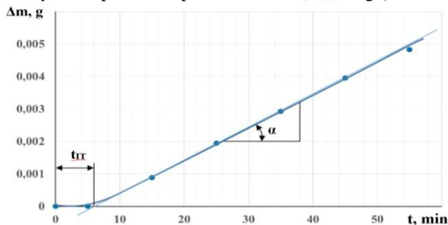
Fig. 7. Curve of solid particle erosion of plastic material
