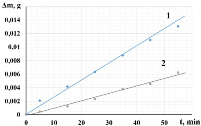
Fig. 12. Results of solid particle erosion tests of compressor blades without coating (1) and with a coating (2) (the tests on the concave side)
