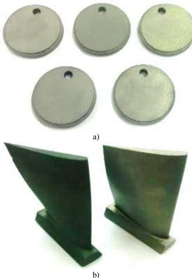
Fig. 2. Experimental samples (a) and rotating blades of the compressor stage (b) made using additive technologies
