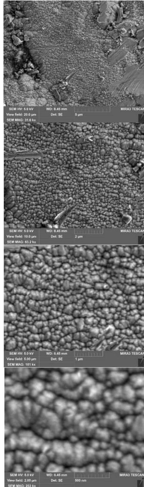
Fig. 11. Surface morphology of Cr-CrC coating Interest
