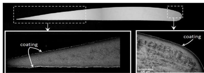
Fig. 8. Cross-section of the rotating blade of the compressor from titanium alloy
