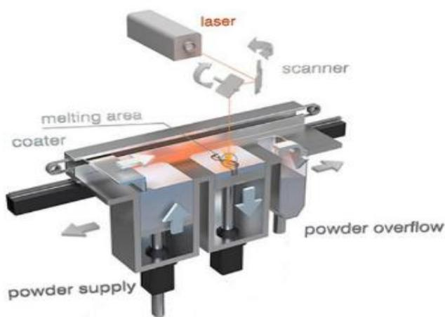
Fig. 1. The scheme of operation of the 3D printer Concept Laser M2 Cusing Multilaser [18]
