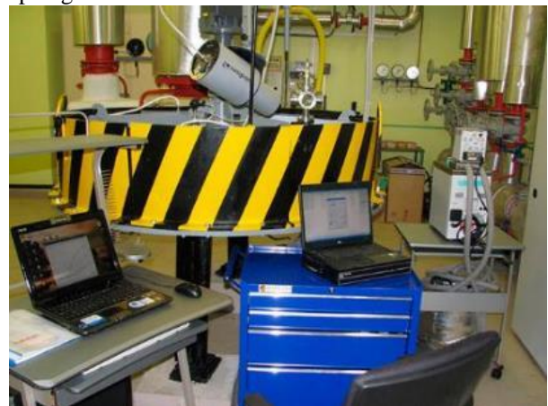
Fig. 6. Erosion–M hydroimpact test rig
