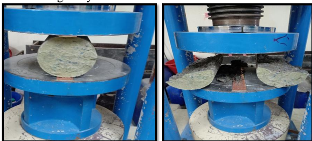
Fig 4 Split Tensile strength test
