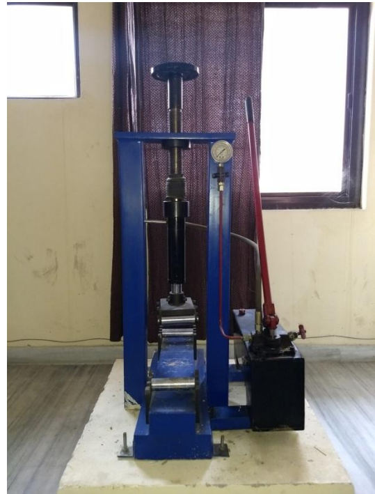
Fig.6 TWO POINT LOAD TEST
