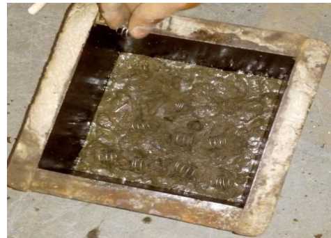
Fig.1 Orientation of Fibers in Cube Mould during Casting
