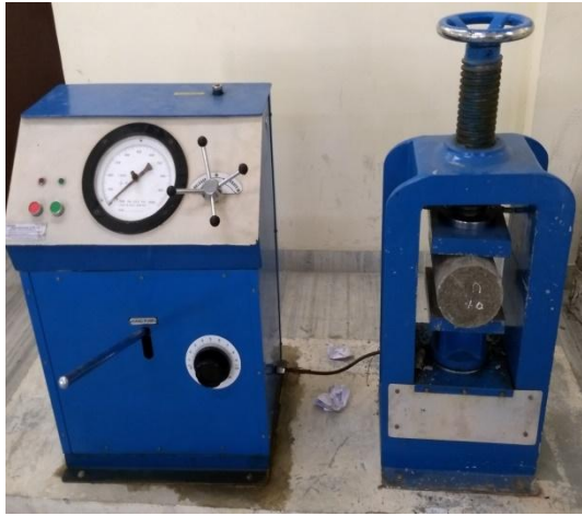
Fig.4 SPLIT TENSILE STRENGTH TEST IN CTM
