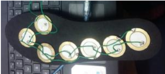
Fig.3 Piezoelectric sensors connected in parallel
