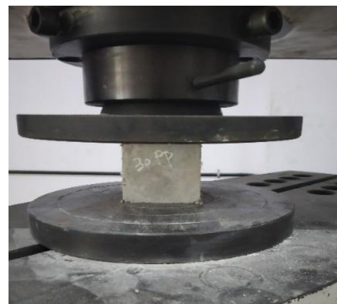
Fig. 1. Compression test on ECC cubes
