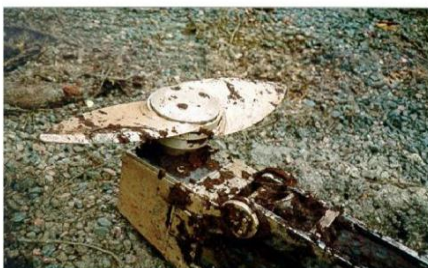
Fig. 10. Deep mixing device for mixing dry mass
