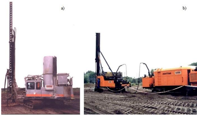
Fig. 7. Mixing unit for deep dry mixing of soil with the hopper, air drier and compressor a); the same with an individual machine for this equipment b)
