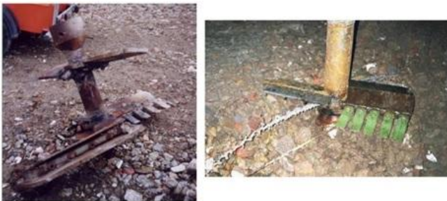
Fig. 9. Mixing devices for deep wet mixing
