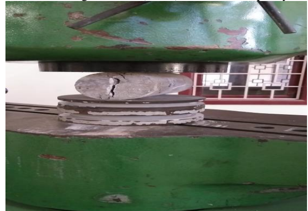
Figure 2 Split Tensile Test
