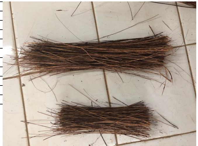
Fig.2: Chopped / cut fibres of length 23.5cm and 16.5cm as per the requirement.
