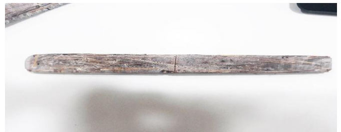
Fig.9: Bending test specimen after testing.
