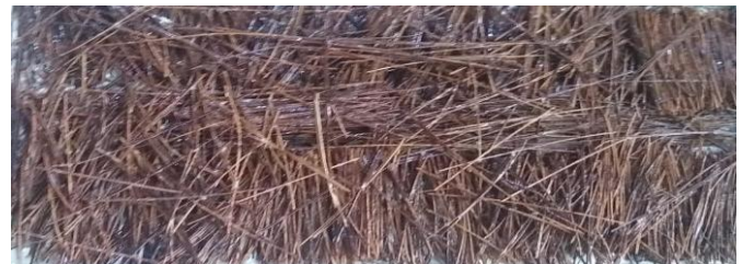
Fig.3: composite after removal from mould.
