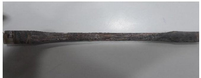
Fig.7: Tensile test specimen after testing.
