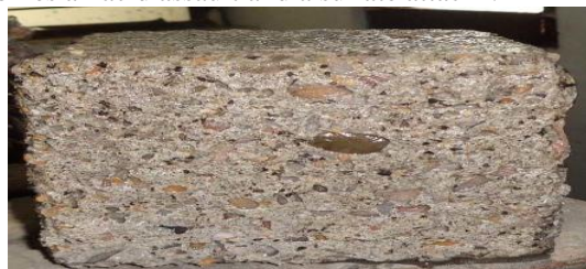
Fig: Acid Attack on Concrete Cube
