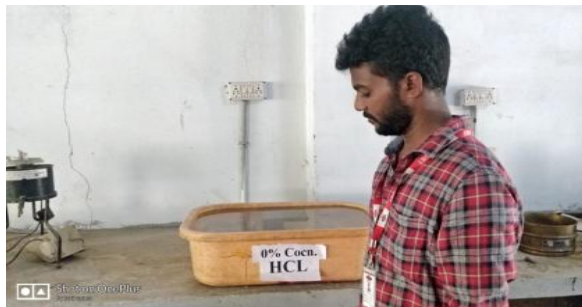
Fig 2. Testing the cube in HCL solution
