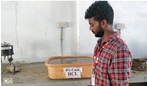
Fig 1.Curing the cube in HCL AND HNO3 solution
