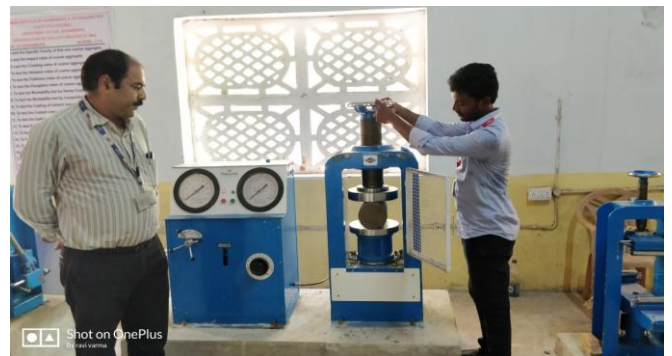
Fig 6. Split tensile testing
