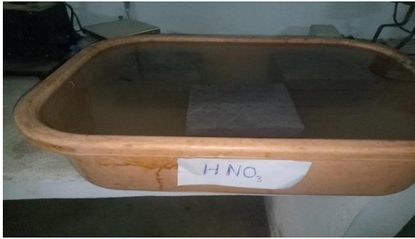
Fig 1.Curing the cube in HCL AND HNO3 solution
