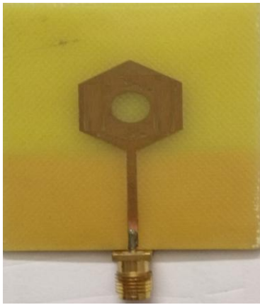
Fig. 10(a) Fabricated Hexagonal Ring antenna top view
