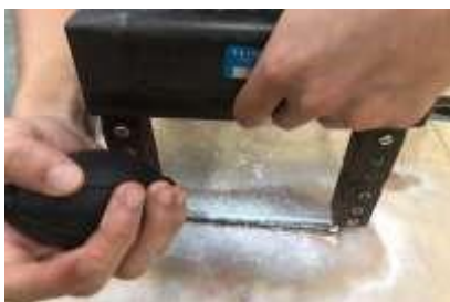
Fig. 5 Bolt Using Dry Method
