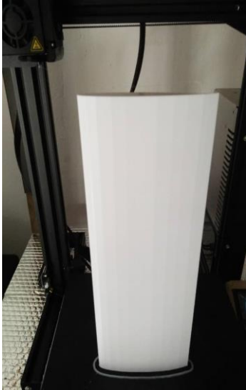
Fig. 11 3D printing process for airfoil with no riblet
