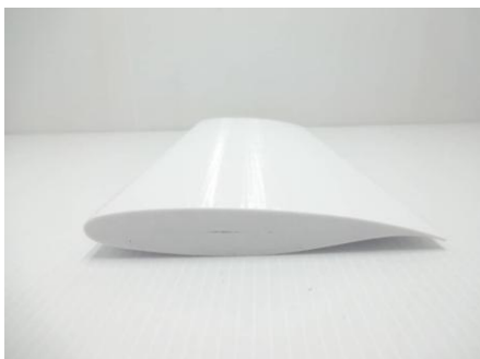
Fig. 13 Wings without riblets
