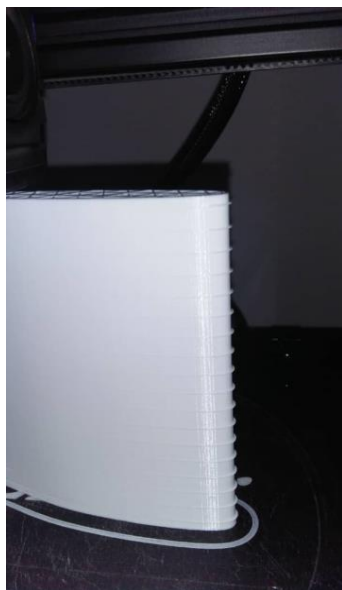
Fig. 12 3D printing process for airfoil with riblets
